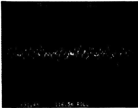
FIGURE 27. PEAK TO PEAK NOISE 0.1HZ TO 10HZ p-p(RTI) = 691.4nV, rms(RTI) = 116.5nV, A_V = 25000
