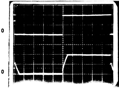
FIGURE 18. VOLTAGE FOLLOWER (A) TEST CIRCUIT (B) RESPONSE TO 20V p-p , 1kHz SQUARE WAVE INPUT
